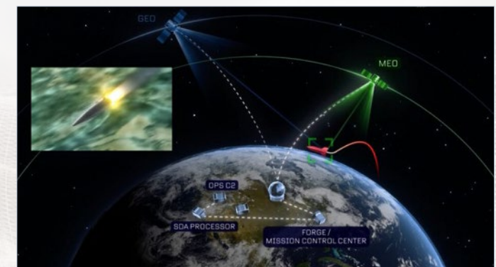
Illustration of GEO and MEO sensor integration with FORGE for missile warning and tracking operations.
