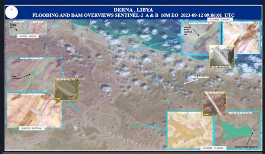
One of many SRT operational planning products delivered in support of the Morocco and Libya disaster response showed dams in Derna, Libya collapsed (left, top right) and at capacity (bottom right)
